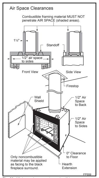
Fig. 20 Minimum clearances to combustibles.
